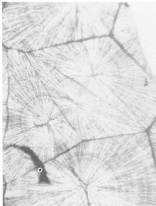
annular ringings, appearing after impregnation/extraction for crystallized PB. The impregnant used is benzyl-neocaprate (reflection micrograph) ( \times 30 ).
