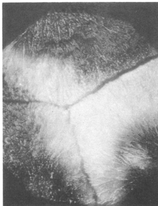
Figure 2 Imperfect joint between three spherulites in PB, T_c = 125^\circ\text{C} (reflection micrograph) ( \times 60 ).
